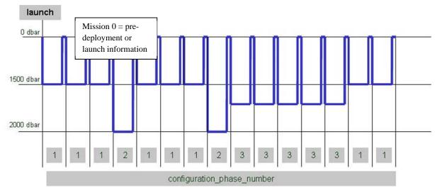
In the above example, there are 3 different float behaviours to record, (with park depth varying between 1500, 2000 and 1700 db). Each of these new behaviours requires a new mission number. This is in addition to the pre-deployment or launch info contained in mission 0:
