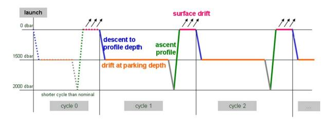
A typical Argo float performs continuously measurement cycle during 3 years or more in the ocean.
